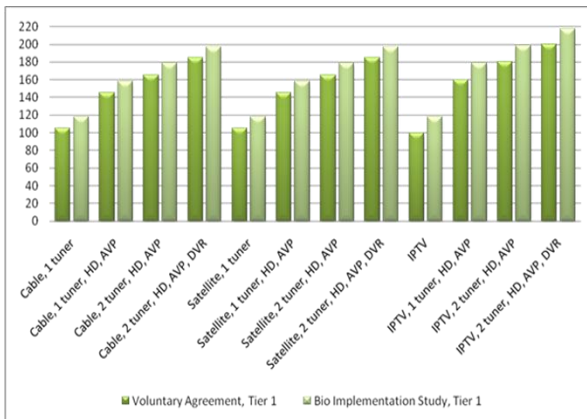
Figure 1: Energy consumption limits – comparison between the VA for CSTBs and Lot 18 preparatory study
